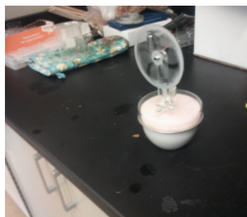
Low temperature stirling engine being powered by pine cone biomass
