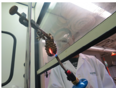
Arianna using mini torch to conduct burn test
