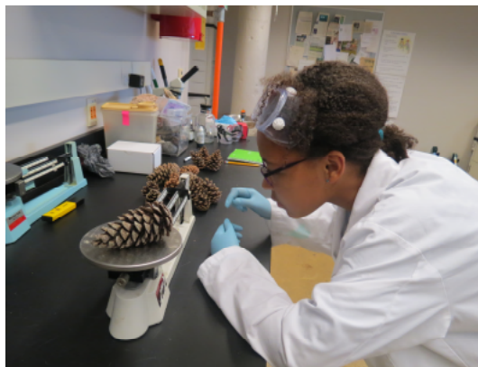
Above: Arianna Fobbs measuring the mass of pine cones in preparation for burn testing
