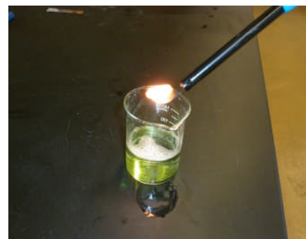
Ignition of biogas while it is stored in low surface tension surfactant aqueous solution
