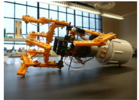
Ventral view of bionic hand prototype showing phalanges and wrist plate
