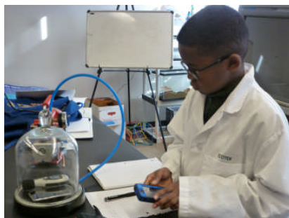
Colin performing sound measurement experiment using bell jar and vacuum pump
