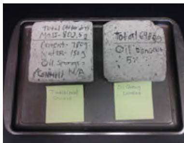
Sample of oil eating cement and traditional cement
